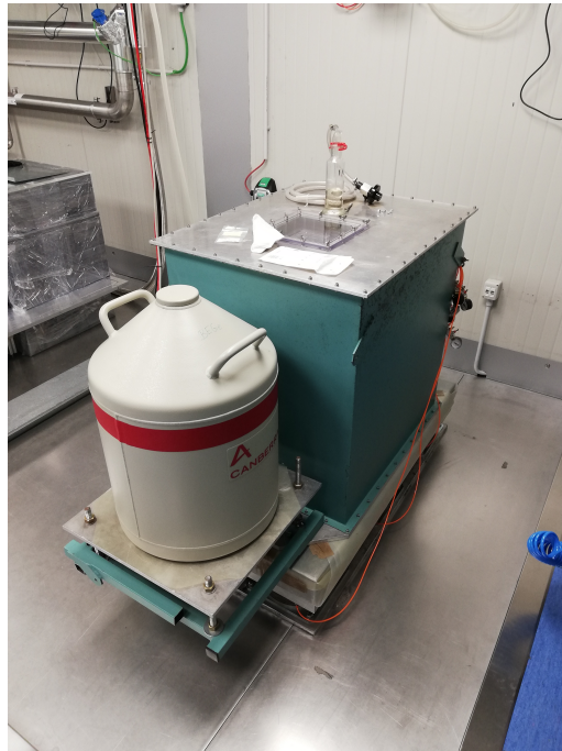
Figure 5: The improved BEGe experimental setup is shown, which is supported by pneumatic suspensions. The whole system is then enclosed by a soundproof box.
