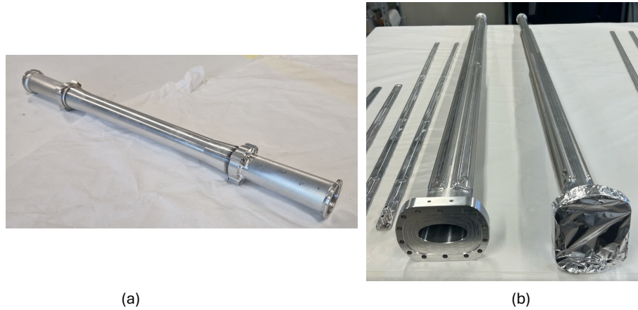
Figure 5: (a) The central chamber fabricated in aluminum with its cooling inlets and outlets. (b): Ellipto-conical vacuum chambers.
