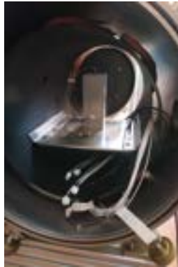
Figure 3: The assembled sample setup: a solid aluminum parallelepiped ( 8 \times 8 \times 20 \text{ cm}^3 ) on its control and support baseplate. With respect to the year 2024 (Figure 2), the wiring is complete and the copper inner shroud has been painted with Aeroglaze Z306 flat black. Credits: INFN-LNF.
