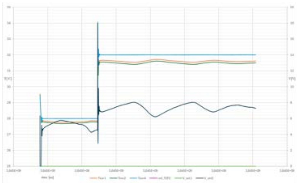
Figure 4: Example of a control plot of the sample controlled to preset temperatures via resistor heaters: left vertical axis: temperature; right vertical axis: voltage; horizontal axis: time (about 6 hours). Credits: INFN-LNF.
