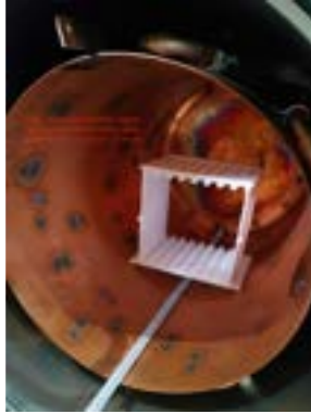
Figure 2: Accessible internal test volume, before recommissioning operations and showing a sample 3D-printed rack for clearance assessment. Credits: INFN-LNF.
