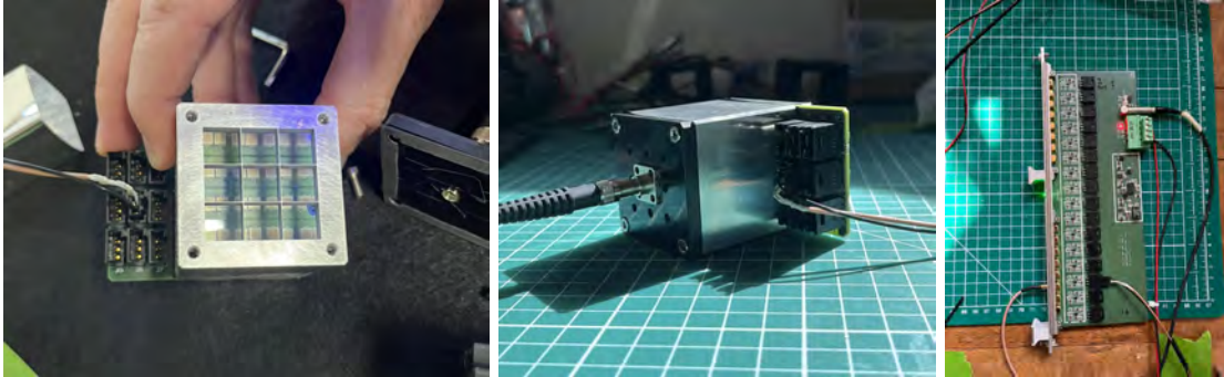
Figure 3: Proto-2, equipped with LYSO crystals for a cosmic ray test prior to beam operations (left, center) and front-end electronics board (right).
