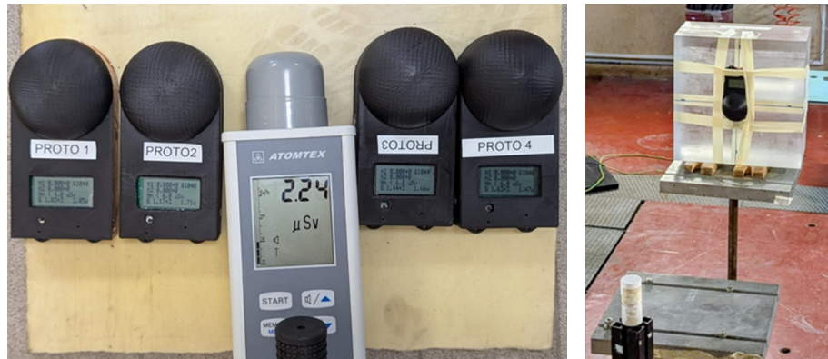
Figure 8: (left) DOIN mini-series of dosimeters assembled, and (right) dosimetric tests at ENEA C.R. Frascati.
