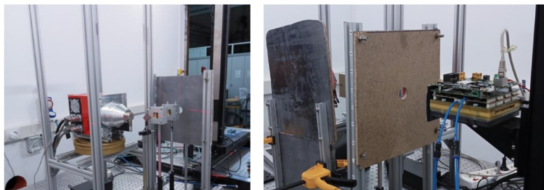
Figure 6: Photos of the experimental set-up at the CNR-ISTP X-ray lab in Milan. On the left, the X-ray tube with the target; on the right the installed side-on GEM detector.
