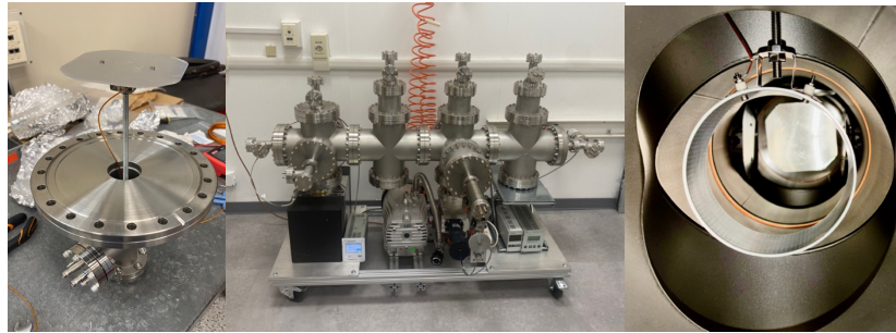
Figure 5: (Center) Overview of the experimental setup to measure the charges emitted by an ion pump and propagating along a pipeline. (Left) Detailed view of one of the metallic screens mounted in the upper flange, facing the ion pump port, and at 90^\circ with respect to the ion pump to collect charges emitted once the ion pump is switched on. (Right) One of the electrostatic rings mounted inside the vacuum line. Both types of screens can be connected to two different picoammeter for current measurements and can be held at a given voltage between -500 V and 500 V.
