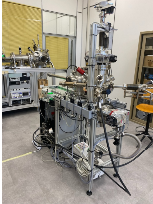
Figure 10: UHV vacuum system for SEY measurements.
