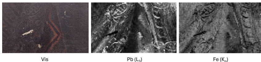
Figure 3: Example of the spatial distribution of Fe and Pb in a 17th-century portrait by an unknown artist, shown alongside the corresponding visible image.
