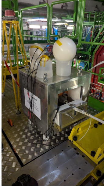
Figure 7: Experimental set-up in CMS cavern with 4 Bonner Spheres, each one containing a couple of SiCs (one bare and one covered with 6-Lithium Fluoride).
