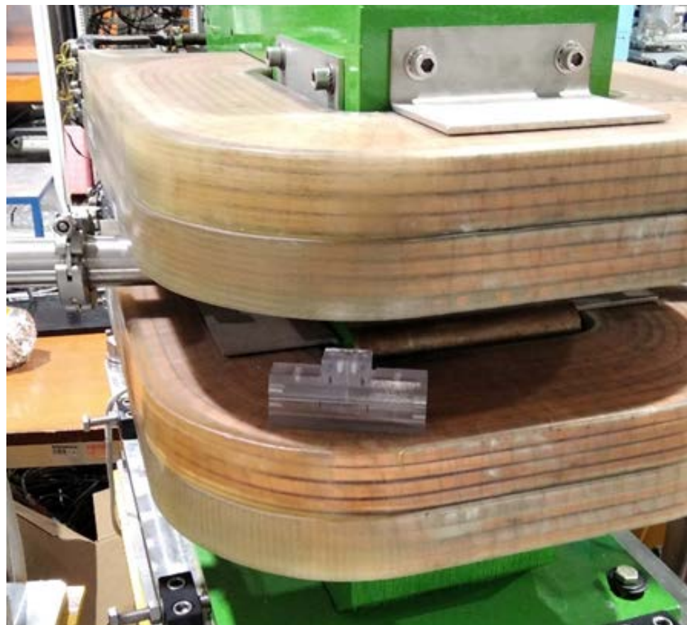
Figure 3: The active bending plasma device compared with a conventional bending magnet.
