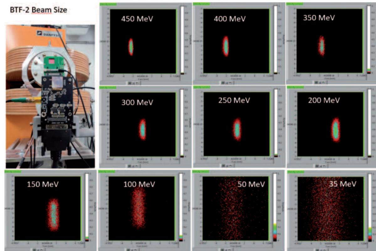
**Figure 4.** Spot size at different beam energies measured at the exit of BTF2 line with the Timepix detector. On the left of the figure the detail of the detector positioning is also shown.
