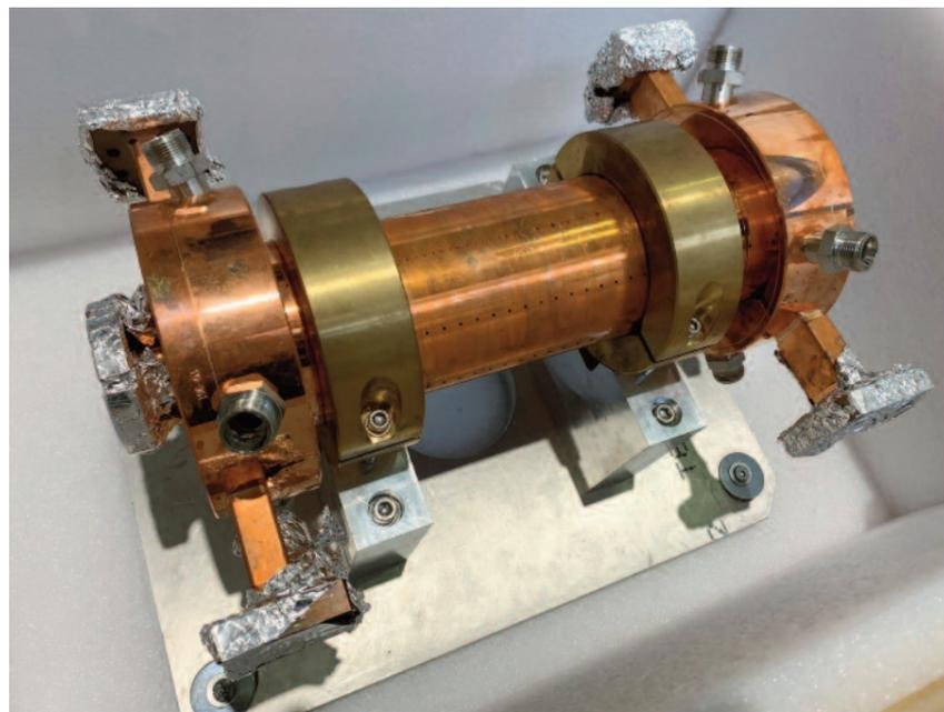
**Figure 7.** X-band accelerating structure prototype, for the CLIC project, provided by CERN.
