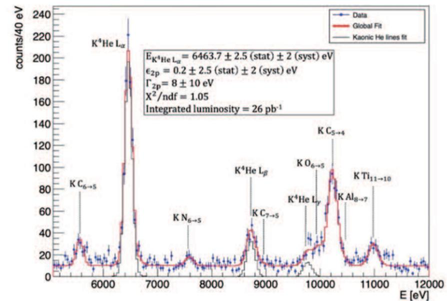
**Figure 3.** Kaonic helium-4 measured by SIDDHARTINO: (red line) fit of the  $K^4\text{He}$  energy spectrum. The  $L_\alpha$  peak is seen together with the  $L_\beta$  and  $L_\gamma$  ones (black lines). The peaks labeled as KN, KC, KAl, KTi (dotted lines) are the lines of the kaonic atoms produced by kaons stopped in the Kapton walls of the target cell and in other parts of the setup.
