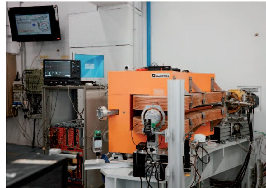
**Figure 3.** The last dipole of BTF2 line. In front of the beam exit window a Timepix detector is mounted. It has been used to characterize the beam during the commissioning phases.
