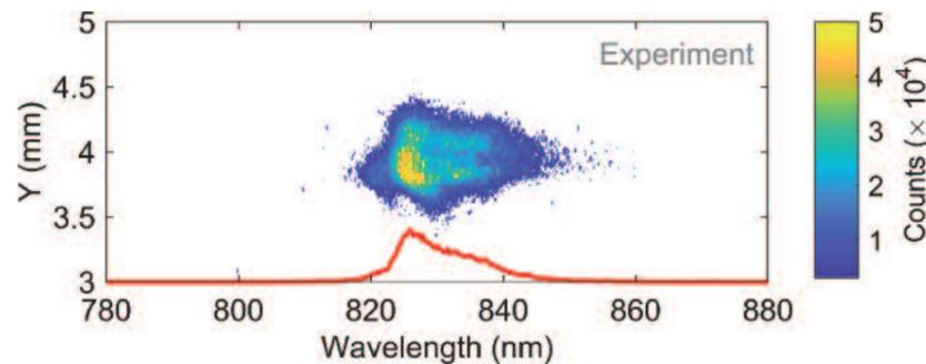
the FEL radiation to a calibrated photo-diode. At the exit of the last undulator the radiation spectrum is also measured with an imaging spectrometer equipped with a diffraction grating and a cooled intensified camera (iCCD). A typical FEL pulse measured with a spectrometer downstream the last undulator is shown in fig.2. The experiment obtained light pulses with maximum energies of 30 nJ.
