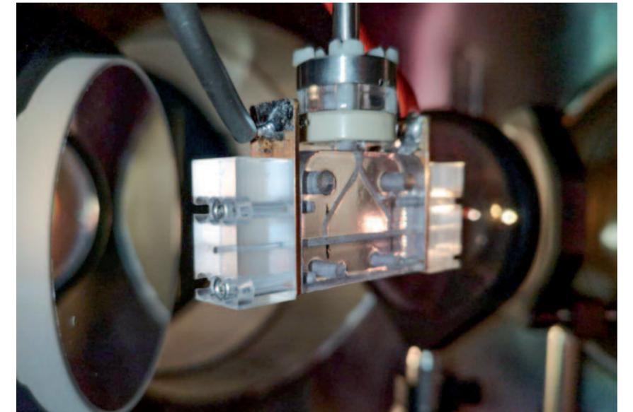
ionizing the hydrogen gas through a high voltage electric discharge (fig. 1). Then the two electron packets have been injected. The first bunch (driver) has the function of exciting the accelerating waves in the plasma which are then exploited by the second one (witness) which is accelerated.
