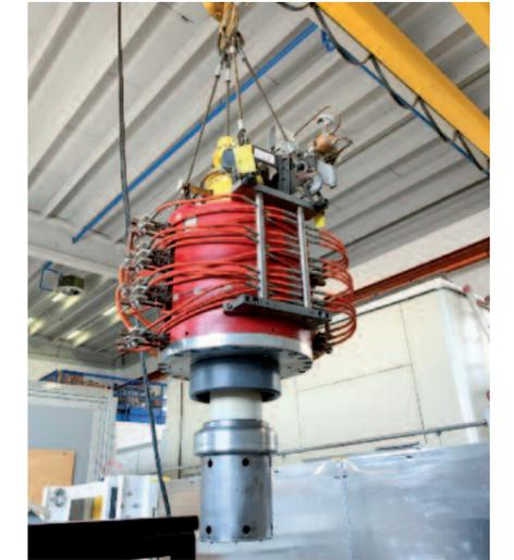
**Figure 5.** VKX8311A klystron during the installation.
