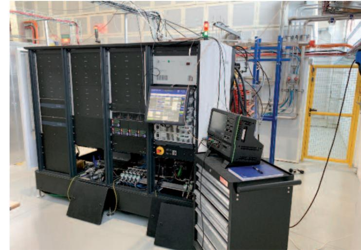
**Figure 4.** Solid state modulator installed near the TEX bunker.
