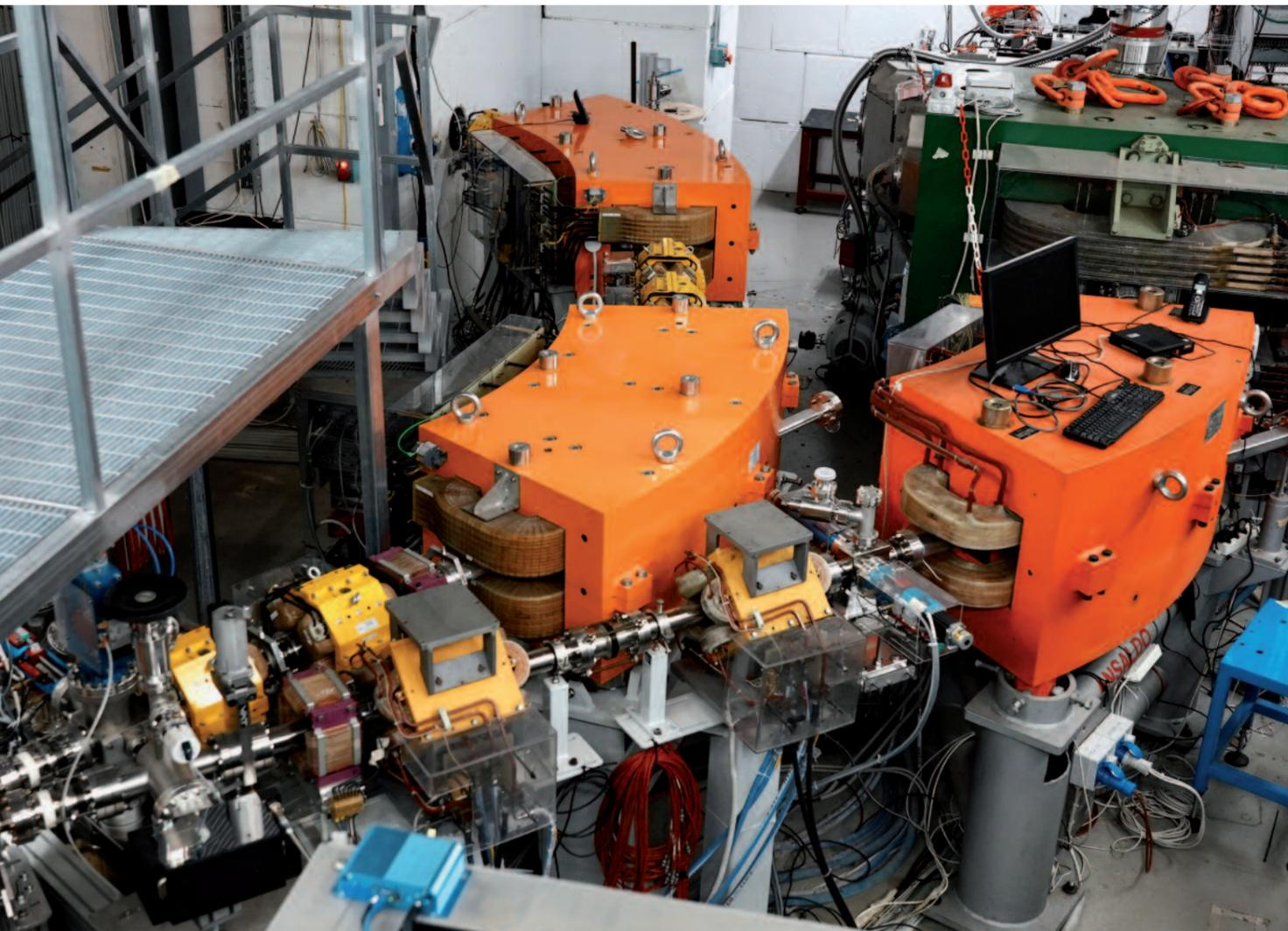
The Beam Test Facility (BTF) is a versatile infrastructure of the DAΦNE accelerator complex. It consists of a magnetic transfer line that transports the LINAC beam in a dedicated experimental area available for external users. During 2021, the upgrade work of the infrastructure has been completed and now two beam lines are available: BTF1 and BTF2. With the new setup, the facility is now able to serve more users and to satisfy different experimental requests.
