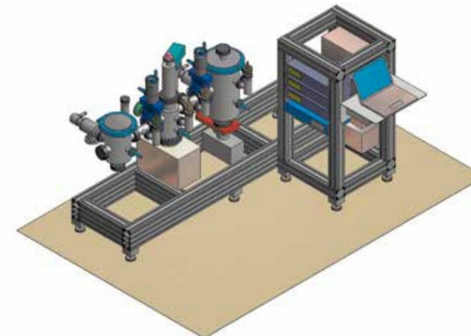
2. A sketch of the degassing measurement system
