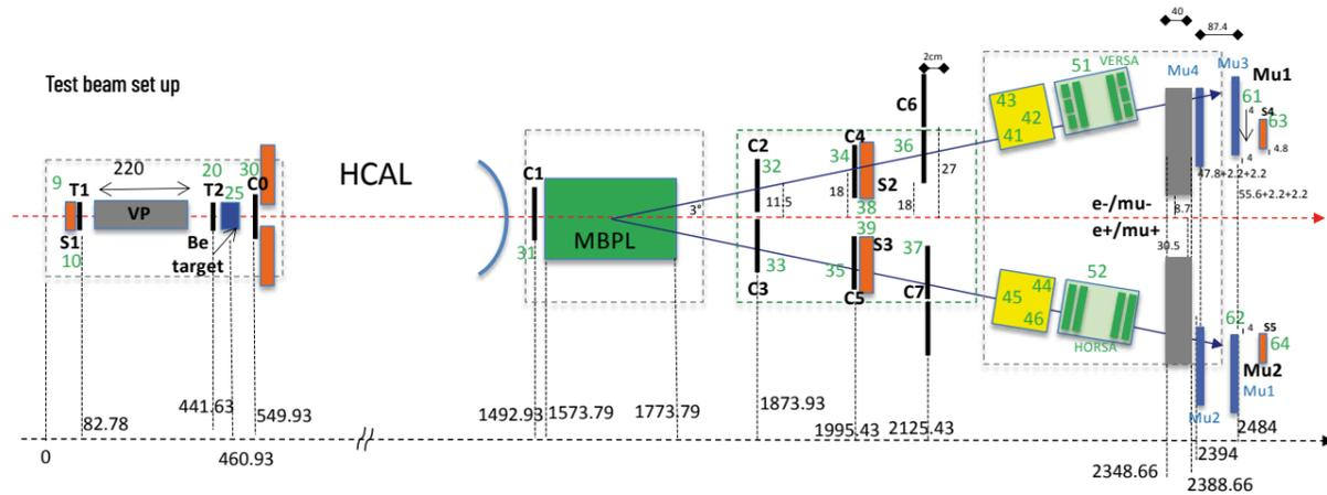
3. (top) North area test beam setup. T1 and T2 are the upstream silicon stations. C0 - C7 represent the downstream silicon stations. Different calorimeters were present in each arm (yellow - lead glass and green Cerenkov). The mu stations are indicated as Mu 1 - Mu4. In orange the trigger scintillators are indicated. (bottom)  $e^+e^- \rightarrow \mu^+\mu^-$  candidate after the full selection of the triggered signal
