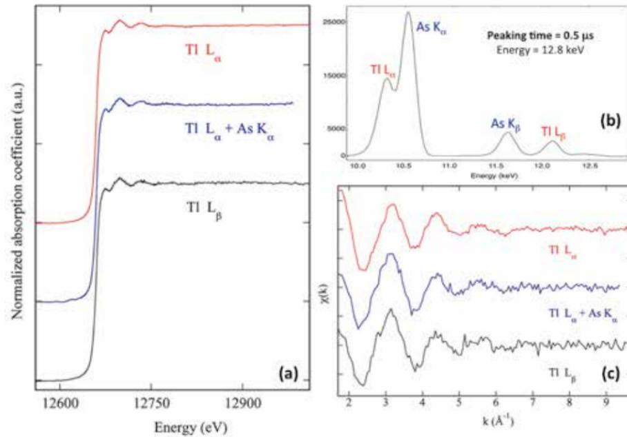
3. (a) XAFS spectra of protochabournéite measured in fluorescence mode using the Tl L<sub>α</sub>, Tl L<sub>β</sub> and Tl L<sub>α</sub> + As K<sub>α</sub> fluorescence lines. (b) protochabournéite fluorescence peaks excited by monochromatic 12.8 keV energy photons. (c) EXAFS or Extended X-ray Absorption Fine Structure spectra extracted from the three XAFS spectra
