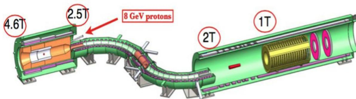
**Figure 6** Layout of the Mu2e experiment solenoidal system: from left to right Production Solenoid, Transport Solenoid and Detector Solenoid. The total length of the experiment is around 25 m.
