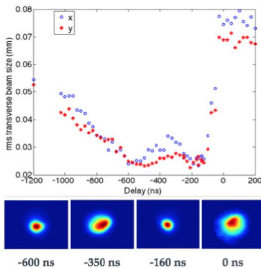
**Figure 16** Transverse beam size evolution as a function of the delay of the bunch with respect to the discharge begin. At positive delays the discharge is off; -550 ns is when the discharge current produces a waist on the screen.
