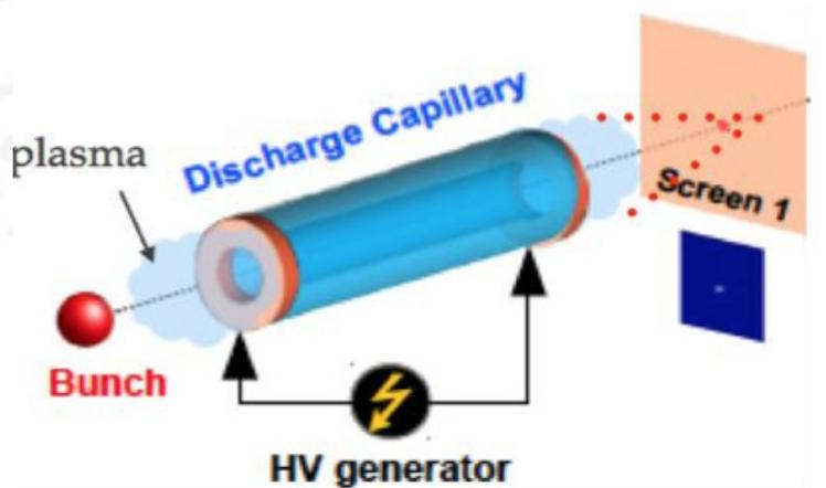
**Figure 15** Layout of a set up to realize an active plasma lens within the SL\_COMB experiment at the SPARC\_LAB (see text for more details).
