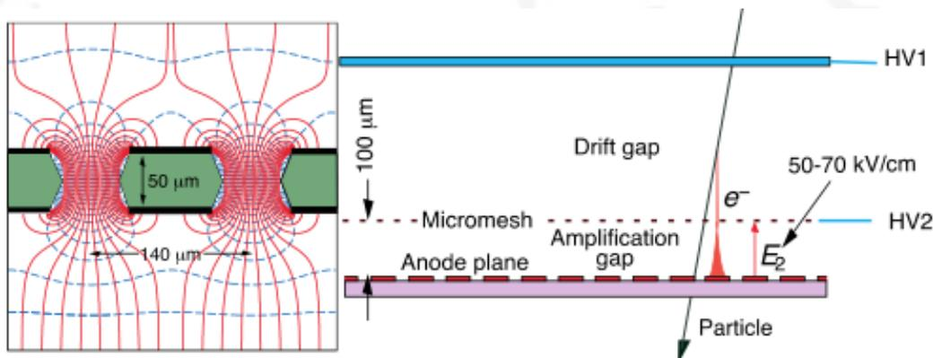
Figure 4 (left) Detailed view of the field lines in a GEM kapton foil; (right) layout of a MicroMegas (from Ref [1]).
