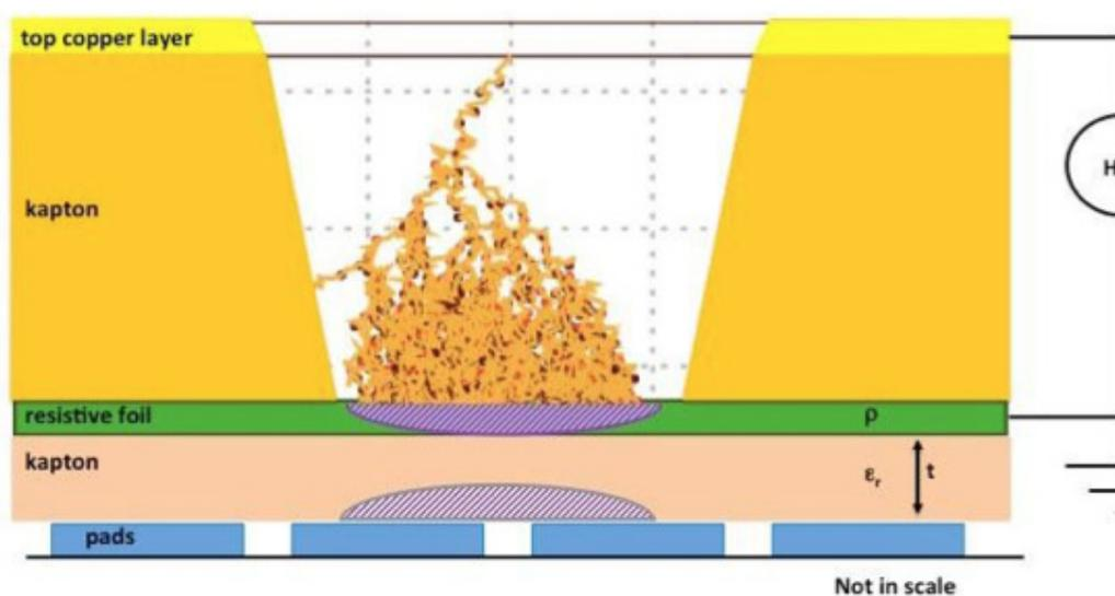
Figure 5 Cross-section of a  $\mu$ -RWELL.
