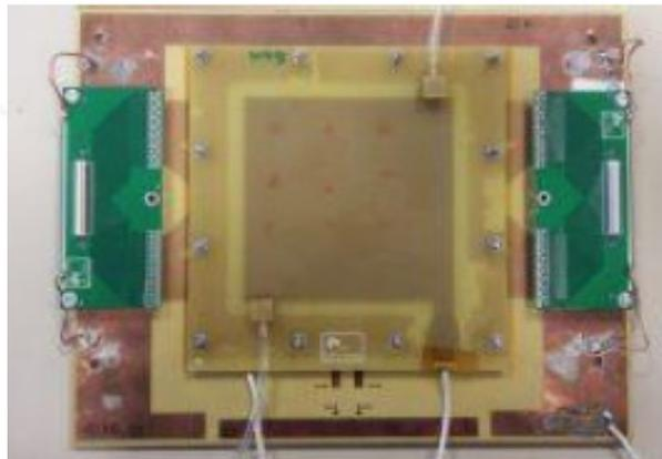
Figure 3 Prototype of a M-RWell.
