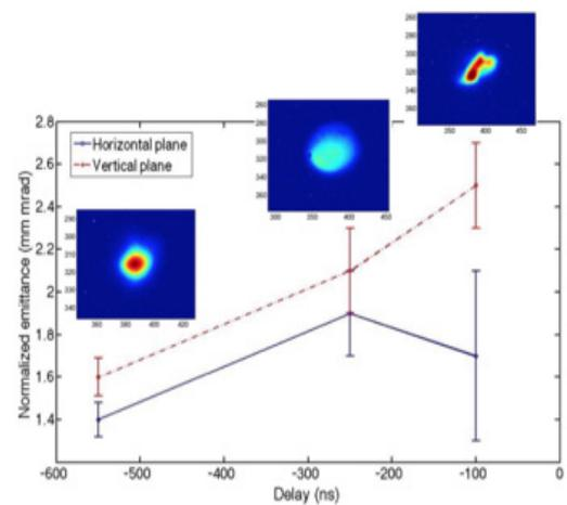
**Figure 17** Beam emittance evolution as a function of the relative time of the discharge.
