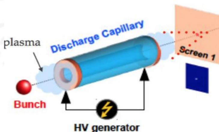
**Figure 15** Layout of a set up to realize an active plasma lens within the SL\_COMB experiment at the SPARC\_LAB (see text for more details).
