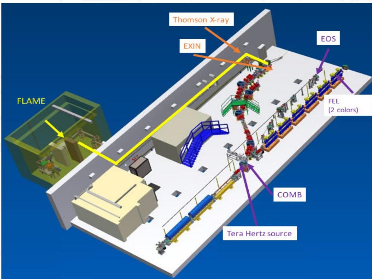
Figure 9 Schematic view of the SPARC facility.
