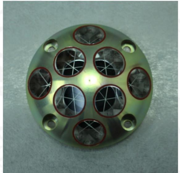
**Fig. 8** Photo of the INstrument for landing - Roving laser Retroreflector Investigations (INRRI) carried on the ExoMars 2016 Schiaparelli entry descent and landing demonstrator module. INRRI has been designed and built at the SCF\_Lab of Frascati.
