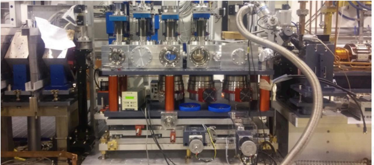
Figure 10 PWFA chamber installed at the end of the SPARC linac.
