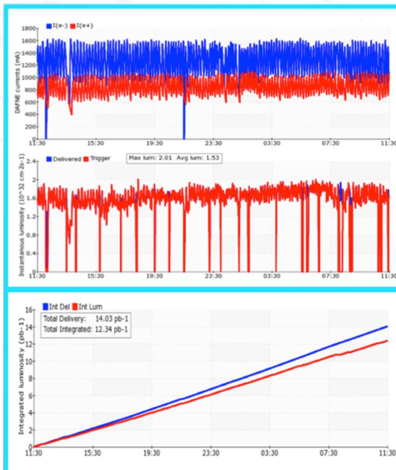
Fig. 3 Plots showing the performance of the DAΦNE collider during one day of operation.
