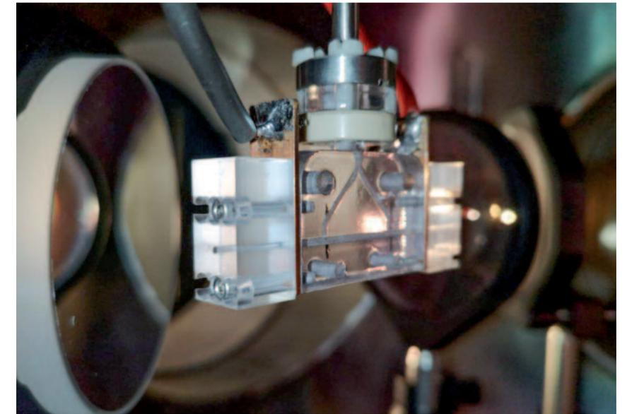
ionizing the hydrogen gas through a high voltage electric discharge (fig. 1). Then the two electron packets have been injected. The first bunch (driver) has the function of exciting the accelerating waves in the plasma which are then exploited by the second one (witness) which is accelerated.
