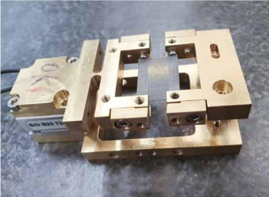
**Figure 1.** The mechanical holder of the bent Silicon crystal of the SHERPA project.
