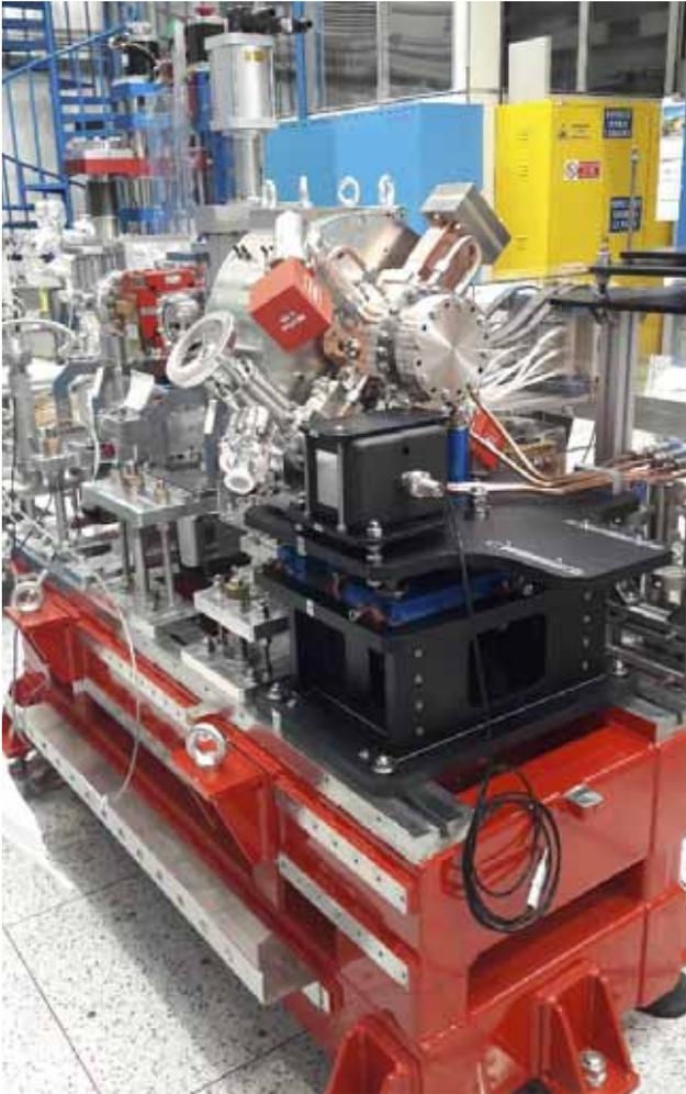
**Figure 2.** The SPARC photo-injector where a laser pulse, hitting a metallic cathode, provides the source for the electron beam.
