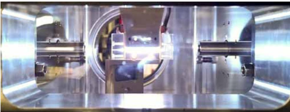
**Figure 1.** Discharge capillary used in the experiment and installed in the SPARC\_LAB interaction vacuum chamber.
