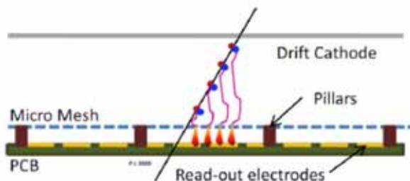
**Figure 1.** Schematic layout of a Micromegas detector.
