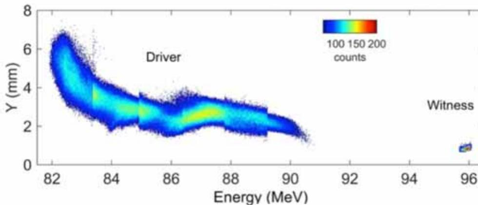
**Figure 3.** Driver (left) and witness (right) after acceleration in 3 cm of plasma. The two bunches had the same energy of 89 MeV before entering into the plasma.
