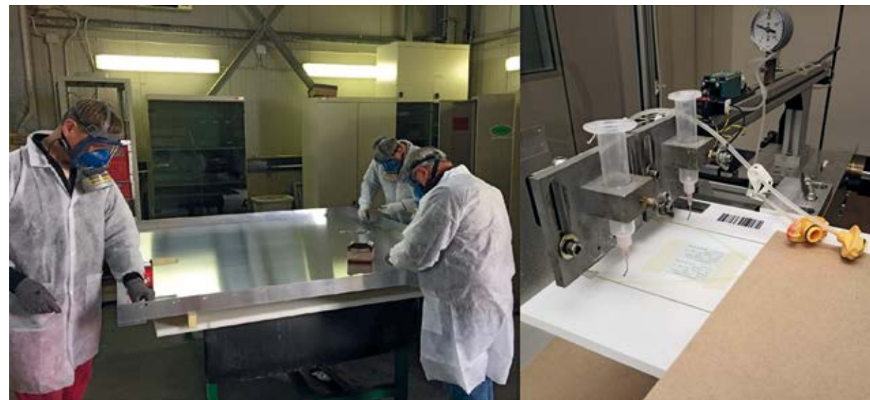
3. (left) Construction of a CRT aluminum case at the construction hall of Bd. 8 of LNF (right) WLS fiber gluing machine located in the clean room of Bd. 28 of LNF
